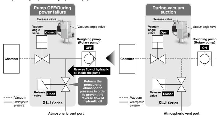
Reduced piping labor due to the built-in release valve structure
