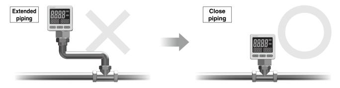
If the product is separated from the original piping, accurate measurements will no longer be possible due to external disturbances such as temperature variation in the extended piping. In addition, increasing the distance from the original piping slows down the temperature transmission and the response.
