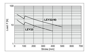
[Stroke] = [Product stroke] + [Distance from the rod end to the center of gravity of the workpiece]
