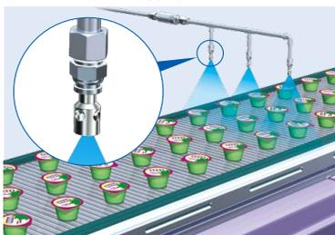
Connects to a restrictor (AS-X21, X214) to allow flow rate adjustment at the nozzle
