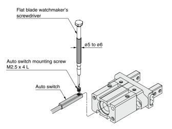
\* Use a watchmaker's screwdriver with a grip diameter of 5 to 6 mm to tighten the auto switch mounting screw.
