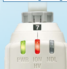
Incorrect high voltage
