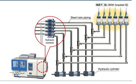
Hydraulic manifold Steel tube piping
