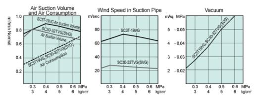
%This data was collected when air valve was on full bore %SC3T-19VG,SC30-32TVG,SC30-32SVG
