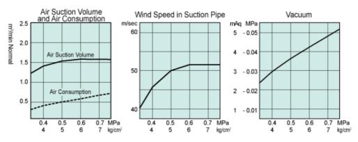
%This data was collected when air valve was on full bore %SC20-32PG(W/F),SC20-32G(W/F),SC30-32SG(W/F)
