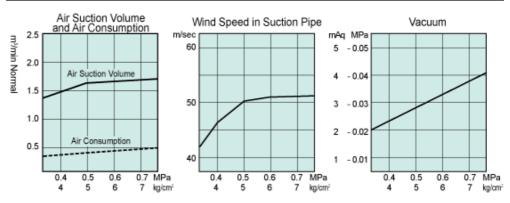
%This data was collected when air valve was on full bore %SC20-32P(W/F),SC20-32(W/F),SC30-32S(W/F)
